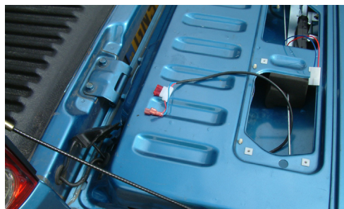
8. Feed cable through grommet
