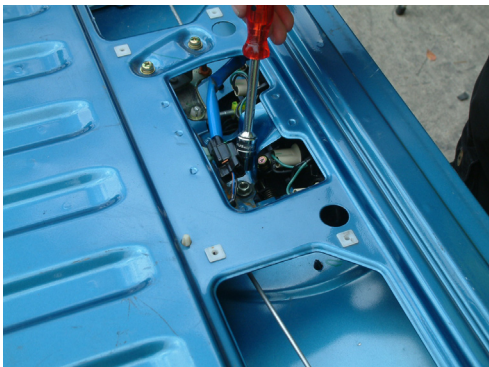
4. Slide bracket into tailgate
