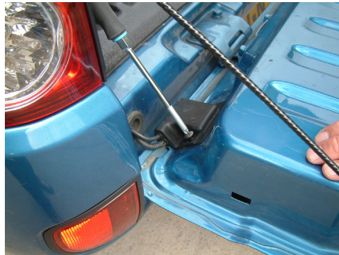
8. Feed cable through grommet
